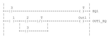
Channels 1, 2, and 3 are the same as for basic motor control. T is the off timer. Notice that this diagram depends on the order of execution of ladder rungs. EQ1 is executed before OUT1\_EQ. The value of EQ1 is initially false because the motor is not running. The start button starts the motor. When the confirm contact closes, EQ1 becomes true and breaks the start circuit, but the confirm contact has closed and the motor stays running.
